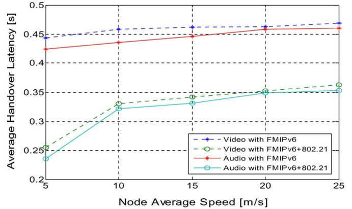
Fig. 6. Average handover latency versus node average speed.
