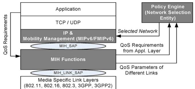
Fig. 5. Cross-layer mechanism for intelligent handover decision making (MN side).
