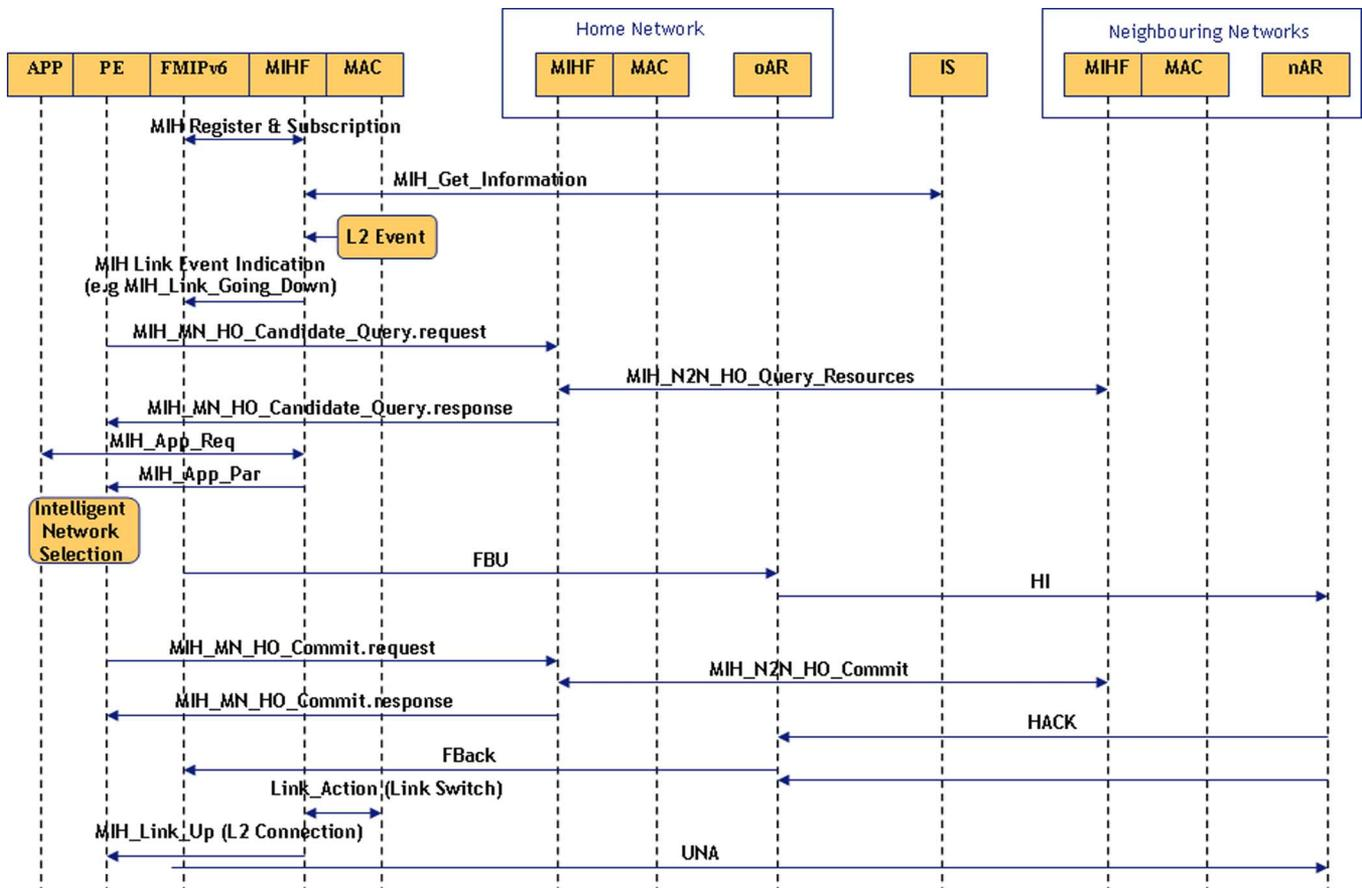
Fig. 4. Message flow in the IEEE-802.21-assisted FMIPv6 handover operations (predictive mode).
