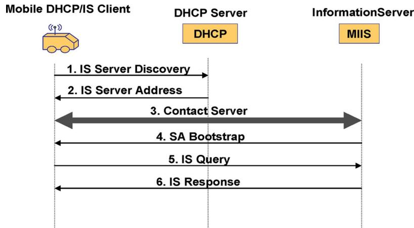
Fig. 3. IS discovery and message exchange.
